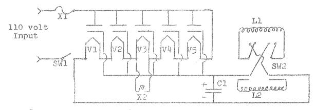
The 2526 tubes are connected in series to produce a 110 volt direct current. The coils should be large enough to prevent overheating. If no other large coils are available, (Cont. in CQC, Page 26)
